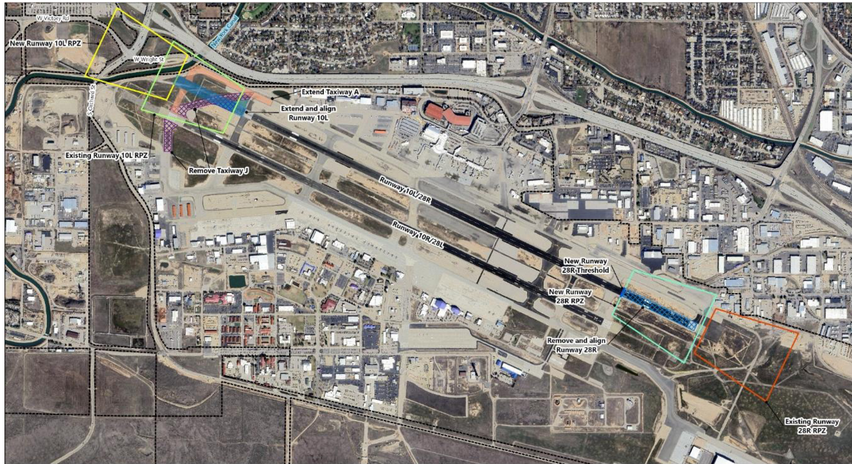
Figure C-1 Alternative 1: Align Runway 10L/28R Thresholds
