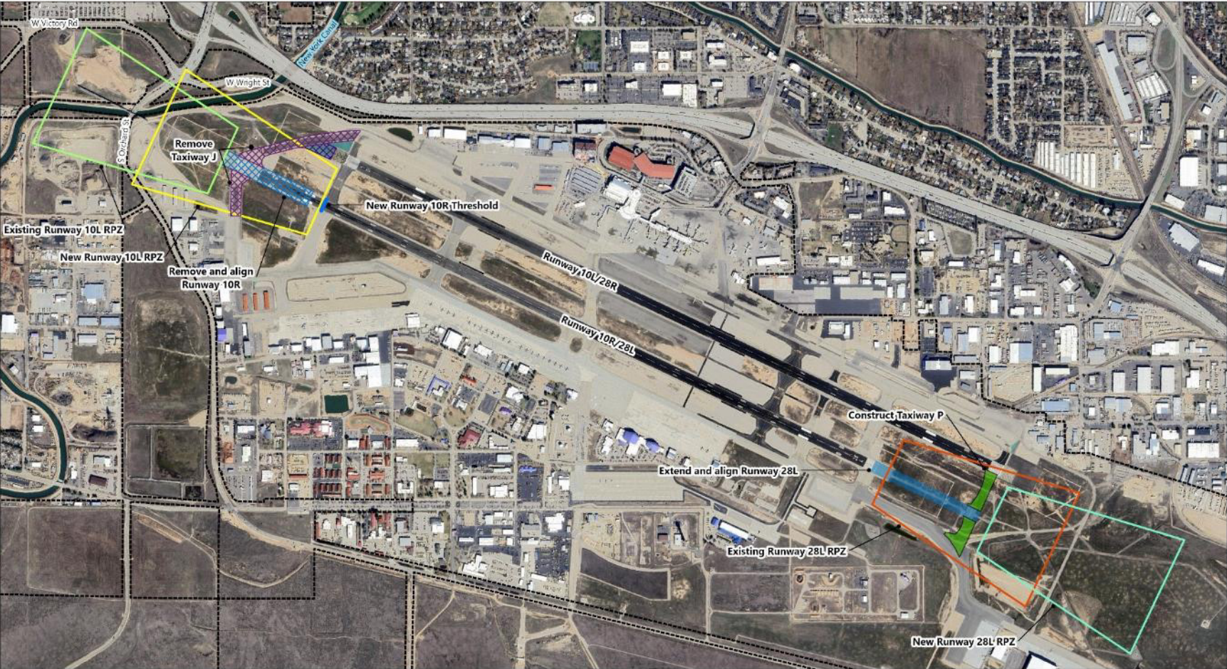
Figure C-2 Alternative 2: Align Runway 10R/28L Thresholds (Proposed Action)
